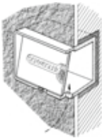
◀ Fig. 2: Installed in an external wall with approx. 4 cm of insulation to prevent loss of heat through conduction
